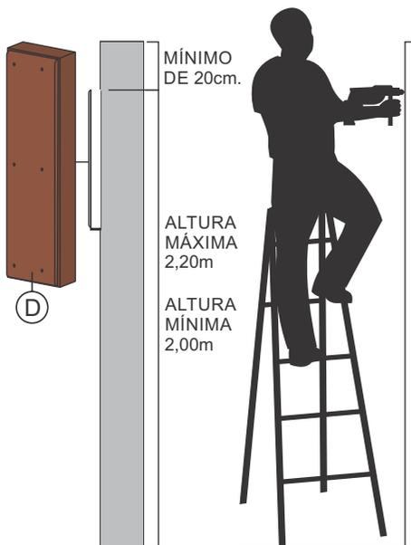
PERFURE A PAREDE DE ACORDO COM OS FUROS DA BASE MANIVELA (D), CONSIDERANDO QUE DEVE HAVER UM MÍNIMO DE 20cm DE PAREDE ACIMA DA BASE MANIVELA (D) E QUE ESTA DEVE SER INSTALADA ENTRE 2,20m (MÁXIMO) E 2,00m (MÍNIMO) DO CHÃO.
