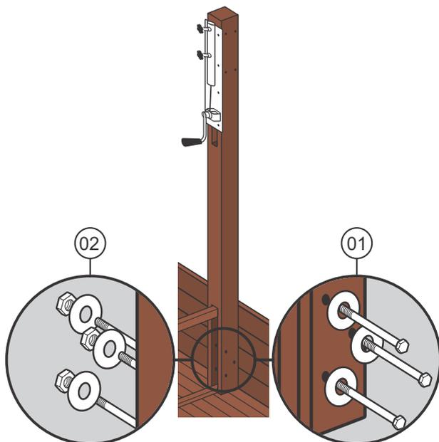
COLOQUE OS PARAFUSOS 3/8 x 5.1/2" (01) COM ARRUELAS NAS PERFURAÇÕES E FIXE COM AS PORCAS E ARRUELAS (02), UTILIZE CHAVE DE BOCA 14mm.
